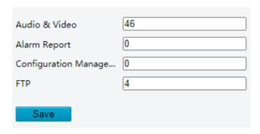
2. Assign a priority level (0 to 63) for each service. The greater the value, the higher the priority. For example, the camera first ensures smooth audio and video in the case of network congestion.
