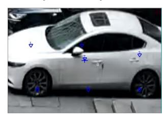
b On the closeup image, find the point that you have marked on the panoramic image, click till the zoom ratio reaches the maximum, adjust the position of the calibration point (small white block) on the panoramic image till it overlaps with the crosshair on the closeup image, and click **Calibrate**.
