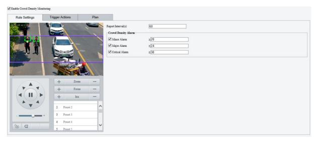
3. A detection box is displayed in the left preview window by default. You can adjust the position and size of it or draw an area as needed. Only one area is allowed.
