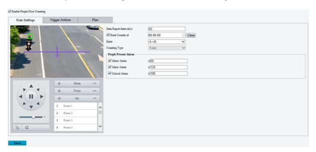
3. A tripwire is displayed in the left preview window. Adjust the position and size of the tripwire as needed or draw a new one. Only one tripwire is allowed.
